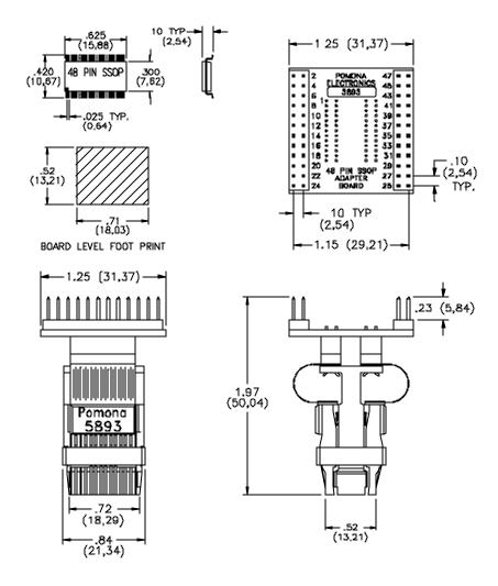
The top interface connects with standard .025" square pins at .100" x .100" spacing. Perfect for use with most logic analyzers.
